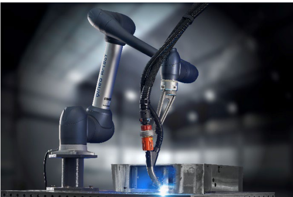
Photo 2: The QINEO ArcBoT relieves employees and ensures consistent, reproducible welding quality.
