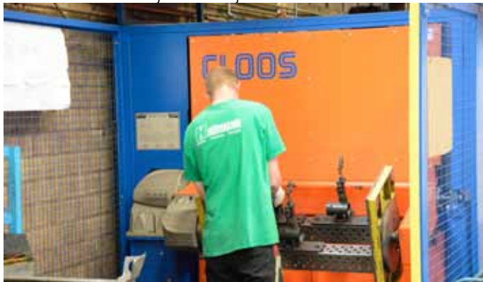
Photo 5: The operator can load one compact cell station whilst welding is performed on the other station on the robot.
