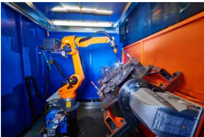
Photo 1: The new welding cell enabled Kuhn to reduce the cycle times for welding the small parts for agricultural machines by 15 percent.
