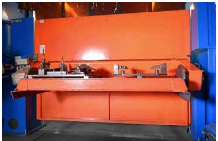
Photo 3: The 2-station positioner consistently brings the workpieces into the optimum welding position.
