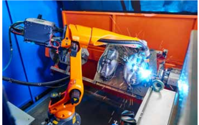
Photo 2: The QIROX QRH-280 compact welding robot is particularly fast and dynamic.
