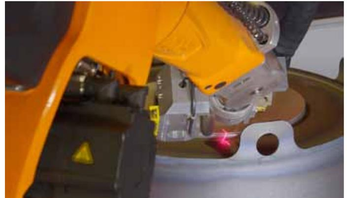
Photo 2: The online laser sensor compensates for component tolerances during the welding process.
