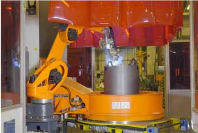
Photo 4: The QIROX robot welds the boiler on both sides.
