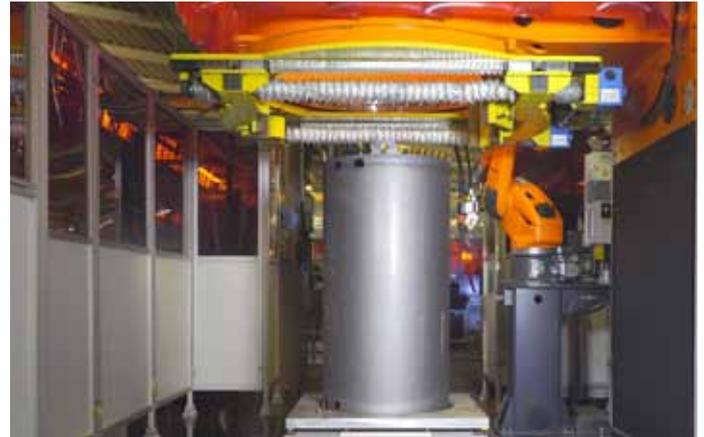
Photo 5: The new CLOOS robot system is able to process a wide range of different boiler types.
