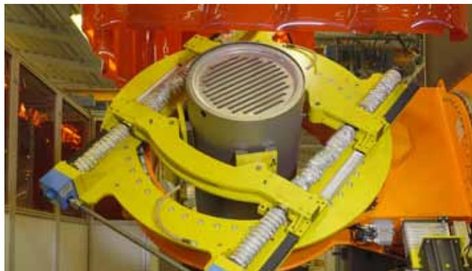
Photo 1: The positioner grips, clamps and rotates the boilers automatically.
